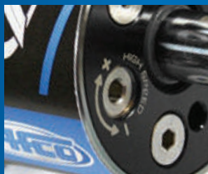
HIGH SPEED REBOUND ADJUSTMENT.
