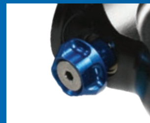
LOW SPEED REBOUND ADJUSTMENT.
