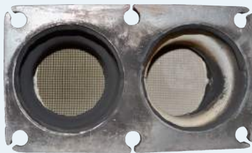
Coolant from a head gasket leak on one cylinder has steam blasted carbon from the Right Inlet. Note the coolant contamination to the substrate.
