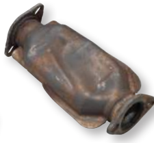
Impact under vehicle crushing converter
