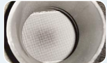
Normal light gray coloration of converter inlet – indicates good mechanical operating condition.
