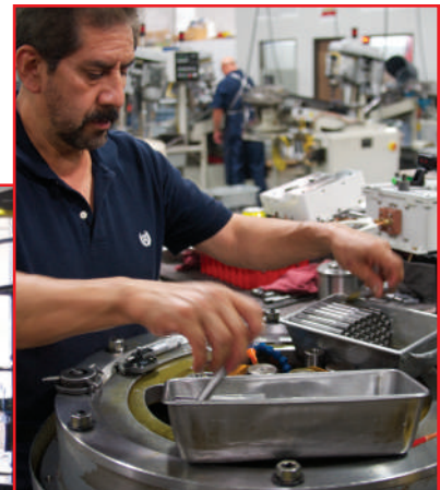
ARP performs the thread rolling operation after heat-treating, which results in a fatigue strength up to 20 times higher than fasteners with threads rolled prior to heat-treatment.
