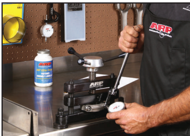
A rod bolt stretch gauge is one of the most important tools a serious engine builder can own. It's valuable in properly setting up a rod for resizing, obtaining the proper clamp load when installed. See page 135 for more information.
