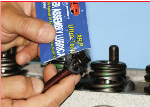
3. Install the head gasket and head, checking for improper fit, binding or misalignment. Make sure all mating surfaces are fully seated. Install the washers on the bolts with the chamfered side of the washer located towards the head of each bolt. Lubricate the washers and the underhead of the bolts with ARP Ultra-Torque fastener assembly lubricant.
