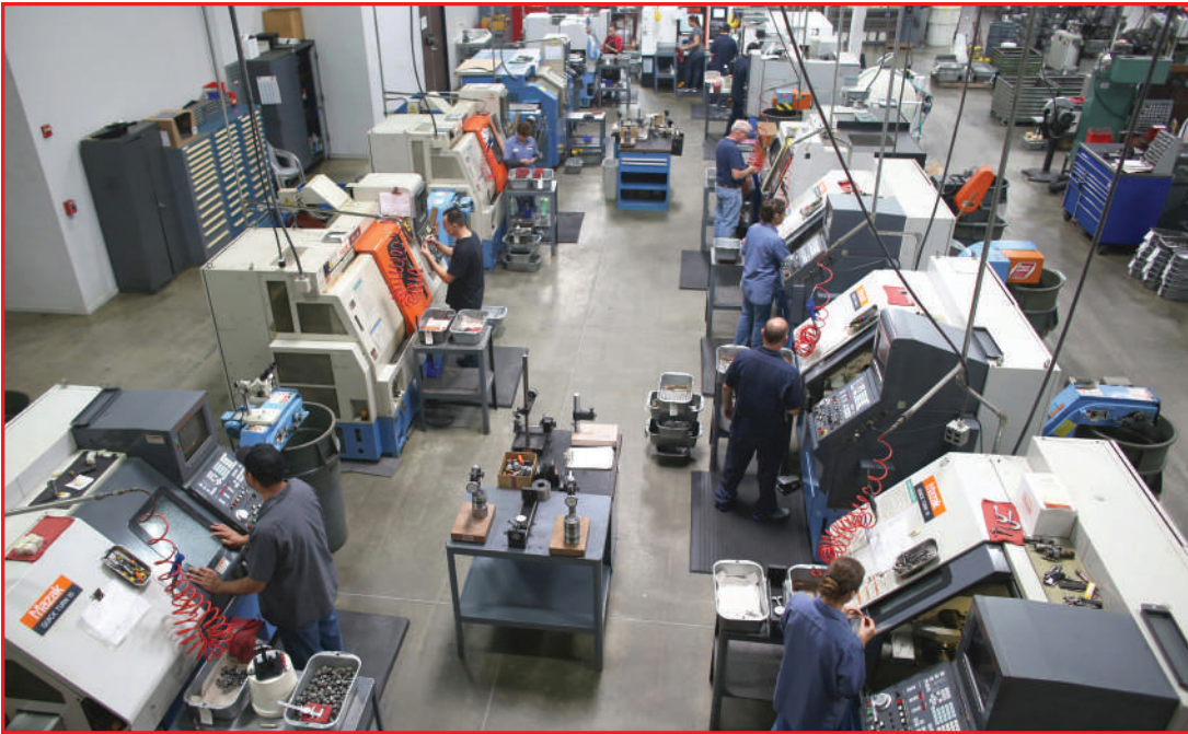
A bank of CNC machining centers are employed at ARP to perform specialty operations.
