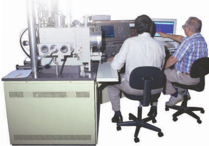
ARP engineers use “Scanning Electron Microscopic” inspection capable of detecting all elements in the periodic table with atomic numbers greater than 5 – permitting the acquisition of high resolution imaging.
