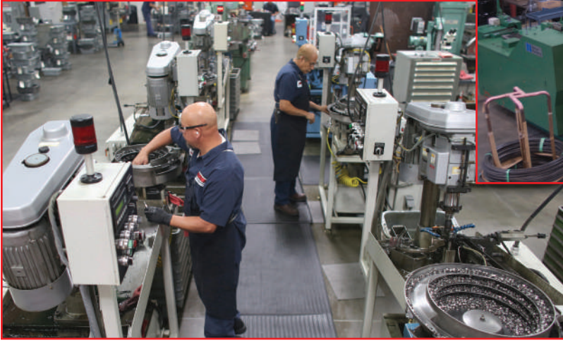
A series of CNC-threading machines are employed by ARP to accurately tap the threads in nuts. Tolerances held are better than aerospace standards.
