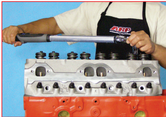
5. Following the engine manufacturer's torque sequence, tighten the nuts to the recommended torque value found on the instruction sheet provided with each kit.
