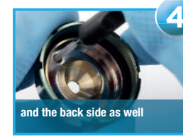
4 Clean also thread of the nozzle carefully with brush
