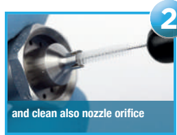
2 Clean the material passage with brush
