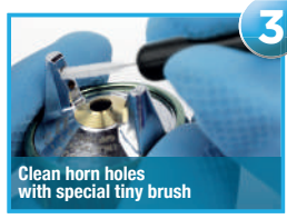
3 Clean tip of the nozzle carefully with brush
