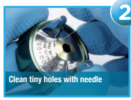
2 and clean also nozzle orifice
