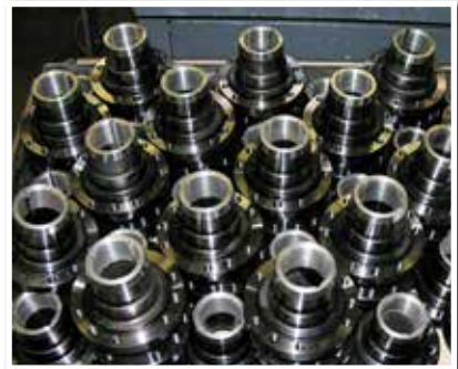
Type 2: Damper with a separate hub and inner shell (Figure 2)
