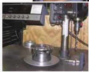
Precision balancing of heavy duty carriers
