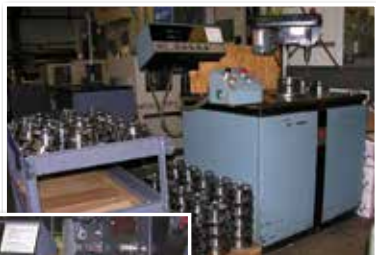
Precision balancing of heavy duty carriers
