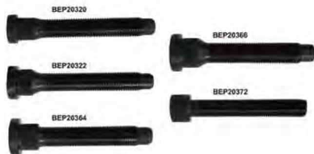
BEP20360 7/16"-20 x 3" Long, .480" Dia. Knurl, Late GM Drum Brake, Applications Hole Size .472"-.479", Quick Start End, 5/PKG. BEP20362 7/16"-20 x 3" Long, .560" Dia. Knurl, Late GM Applications, Hole Size .552"-.559", Quick Start End, 5/PKG. BEP20364 1/2"-20 x 3" Long, .615" Dia. Knurl, Ford Disc Brake and Mopar Front, Applications Hole Size .606"-.613", Quick Start End, 5/PKG. BEP20366 1/2"-20 x 3" Long, .685" Dia. Knurl, Chrysler B, E Body Rear with 1/2" Studs, Applications Hole Size .676"-.683", Quick Start End, 5/PKG. BEP20372 1/2"-20 x 3" Long, Screw-in, Fits all Aftermarket Axles with 1/2"-20 Threads, 5/PKG.
