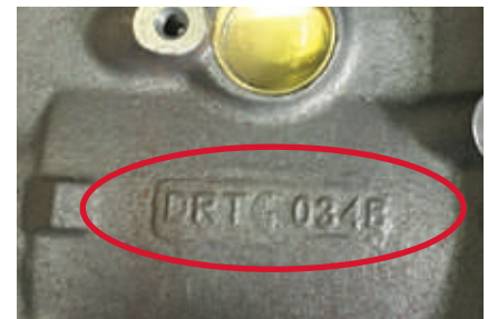
MRK IV, Gen V and Gen VI blocks with water between the bores are identified by a B suffix on the casting number.
