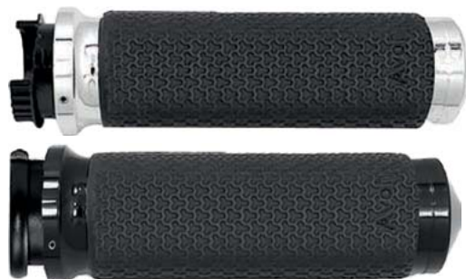
Complete with interchangeable throttle cams
