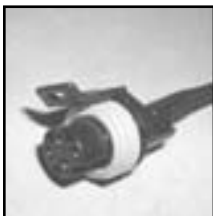
2890F GM Oil Pressure Switch Connector 1987-95 GM 12085539
