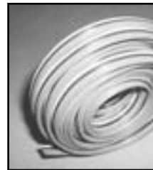
2522F 4-Way Trailer Ribbon Wire Four bonded. Parallel primary, color-coded wires (green, yellow, brown & white) in 25 ft. length, 16 AWG.
