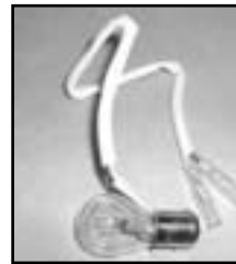
2560F 1157 bulb, adapted w/leads for easy tap-in from tow vehicle tail light.
