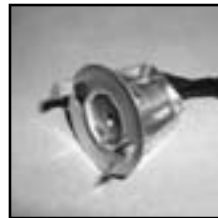
2561H Universal Double Contact Socket Assembly Doublecontact socket w/spring clip mount for park, stop & tail, license plate, instrument panel assembly. Fits 7/8" to 1-1/8" hole. Lamp #198, 1016, 1034, 1154, 1157
