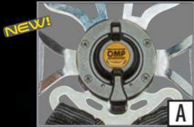
Lightweight buckle with anti-unwitting opening system. FIA 8853/2016
