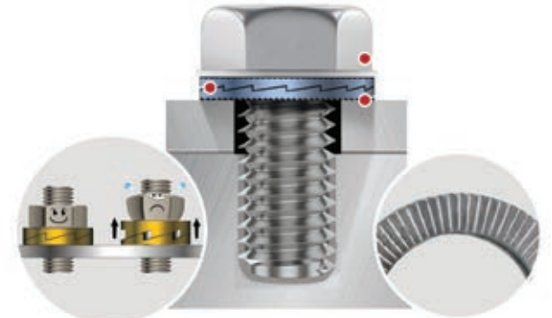
Wedge-Locking Cams Prevent Bolts From Loosening with Engine Vibration
