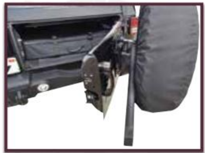
Rear Gate and Tire Carrier joined together to work in unison.
