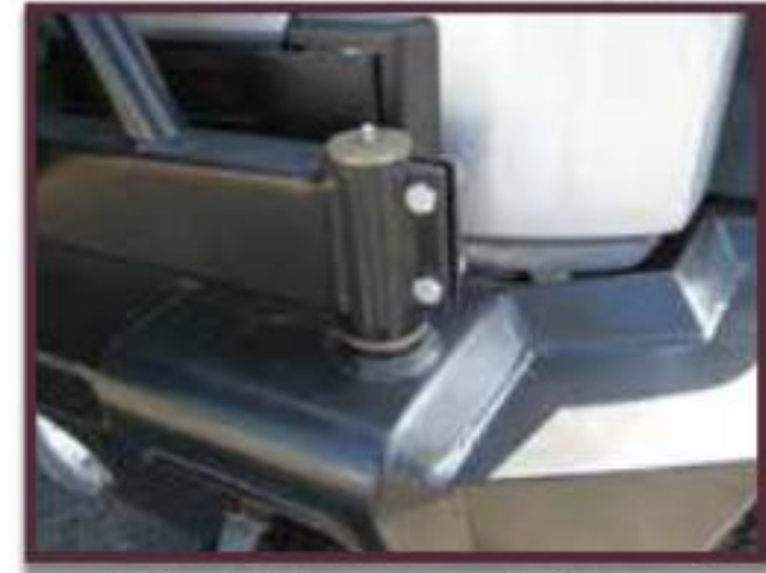
Adjustable, easy swivel hinge with grease fitting.
