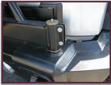
Adjustable, easy swivel hinge with grease fitting.
