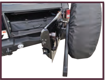
Rear Gate and Tire Carrier joined together to work in unison.
