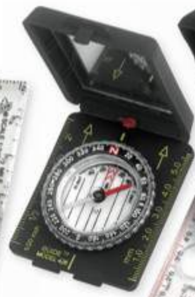
429 SILVA GUIDE 426 COMPASS , 2° graduations and declination scale, sighting mirror, floats in water, lanyard**
