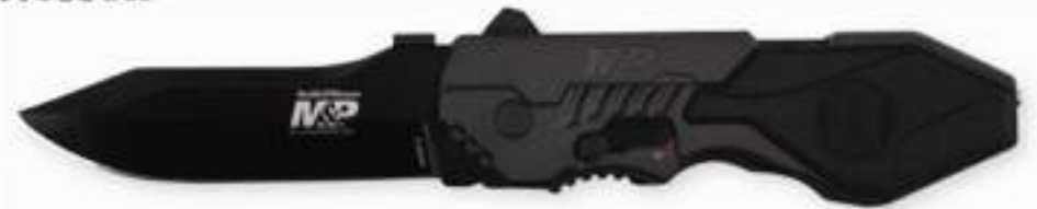
3317 SMITH & WESSON M & P ASSISTED OPENING KNIFE (SWMP4L), 3.6" 4034 stainless steel drop point blade w/black coating, 8.6" overall, black aluminum handle w/rubber outlay, liner & safety lock, pocket clip*
