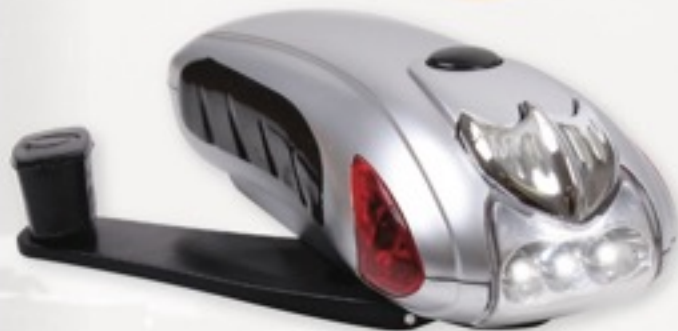
548 WIND UP LED FLASHLIGHT , 3 bright white LED lights, 2 red side lights, 2 settings for brightness, flashing light for emergency use, 1 minute of wind-up generates 30 minutes of light, great for power outages, camping, etc.
