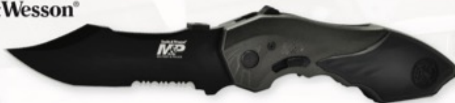
3364 SMITH & WESSON MILITARY POLICE ASSISTED OPENING KNIFE (SWMP5LS), 3 1/2" 4034 stainless steel combo edge blade w/black coating, aluminum handle, glass breaker tip, liner lock & safety lock, pocket clip
