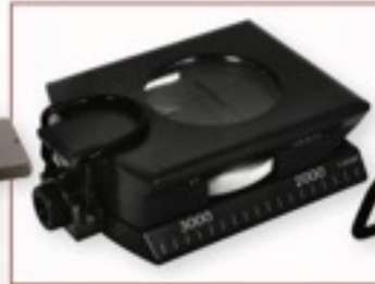
ROTHCO DELUXE MILITARY MARCHING COMPASSES , features: zinc alloy case, inclination scale, side ruler, level, magnifier, green fluorescent North arrow, 360° and mils. circular scale
