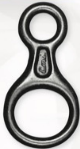
275 FIGURE 8 RING , #1 forged aluminum ring for descending or belaying, 5 1/2" x 3", 10,000 lb test
