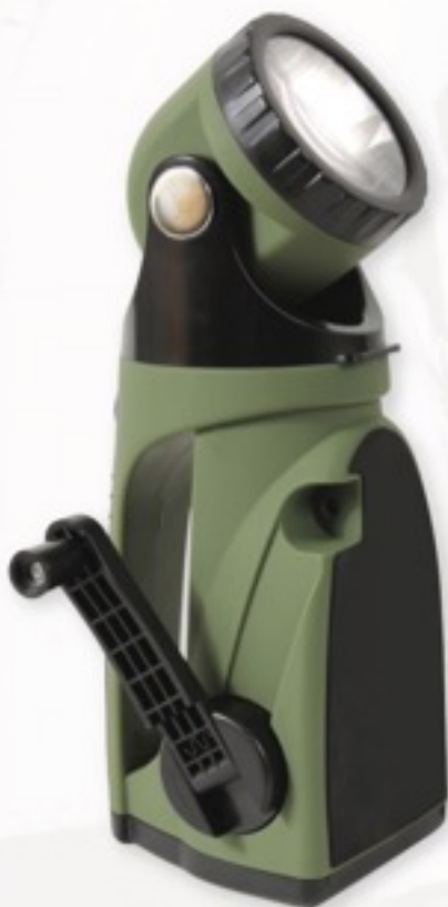
898 ROTHCO O.D. 9-BULB LED HAND CRANK SWIVELHEAD FLASHLIGHT , features: ABS plastic, charging and fully charged indicator lights (charger not included), 180° swivel head, magnetic base, 3 lighting modes: single white LED, 5 white LED's & 4 red flashing LED's for emergency use, 1 LED runs continuously up to 30 hours on a full charge, 5 LED's up to 6 hours & flashing mode up to 60 hours, great for camping, survival or at home
