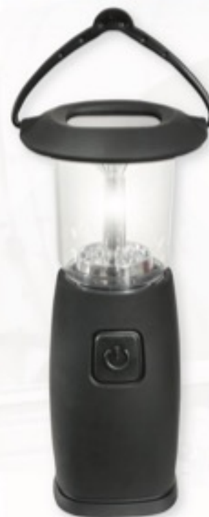
80007 6-BULB LED SOLAR/HANDCRANK LANTERN , ABS plastic, wind up or charge in direct sunlight, 2-function switch for 3 or 6 LEDs, 16 hours in sun will provide up to 6 hours of use, 1 minute of hand cranking provides up to 20 minutes of use, includes Ni-MH rechargeable battery, 7¼" x 3¼"
