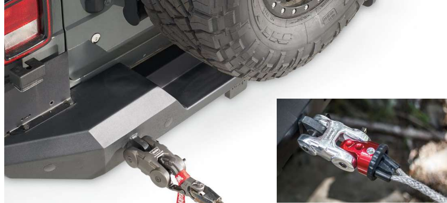
Hyperlink direct-connection to thimble-type rope attachment. No need for additional shackles.
