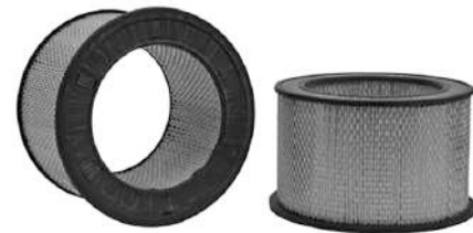
Round air filter -- plastisol ends with "flap" on one end. Perforated metal inner and outer bodies with cellulose media.
