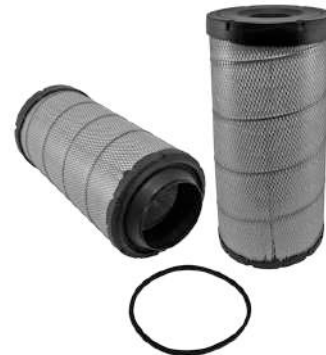
Radial seal HD air filter with urethane end caps -- bottom end has raised sealing area - top end has "dump hole."
